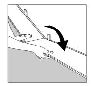
**3.** At the end of the first row: Leave a gap of  $\frac{1}{2}$ " / 10 mm to the wall to avoid any damage while installing your floor and measure the length of the last plank to fit. Insert the short side and tap it closed, using a pull bar.
