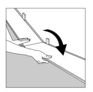
3. At the end of the first row: Leave a gap of ½" / 10 mm to the wall to avoid any damage while installing your floor and measure the length of the last plank to fit. Insert the short side and tap it closed, using a pull bar.
