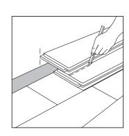
7. Holes for pipes: Measure the diameter of the pipe and drill a hole that is 3/4" / 20 mm larger. Saw off a piece as shown in the figure and lay the board in place on the floor. Then lay the sawed-off piece in place.
