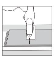
4. Starting second row: Rows can be started with end cuts if the cut plank is at least 12" / 30 cm long. If end cut is used for subsequent row a stair step pattern is established. Starting planks of random lengths will create a more aesthetic random stagger. Short end joints must not be closer than 8" / 20 cm to each other.
