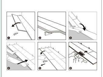
**Tip**: After finishing the installation of every row, use a tapping block or cutoff and a rubber mallet to gently tap the planks into the click of the previous row to make sure they are tightly clicked together and make sure there is no gap between the long side of the planks installed. Any gapping can compromise the whole installation.
