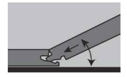
8. For the next piece, engage the angle lock but do not press down until it is directly over the top of the right hand end lock of the first piece. Once it is in position, press down firmly to lock both the ends and the length of the planks. Continue this way whilst using your tapping block and mallet on each plank to ensure correct engagement of the locking system.
