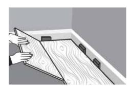
7. Commence locking in the second row by angling in the starting piece at approx 30°. Press it down until it clicks into place. Use your mallet and tapping block to ensure correct engagement of the locking system.
