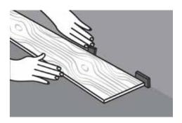
5. For the first row, position the left end lock of the second plank directly on top of the right end lock on the first plank then firmly press down to engage the *Best Lock Ex-treme*<sup>®</sup> locking system. The lock is engaged when you hear a click then lightly tap with your mallet to ensure the lock is engaged correctly.
