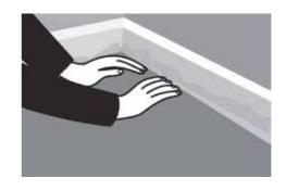
2. Tape the joins with vapour proof tape or the joiner provided.
