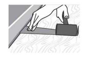
11. Once you have finished the final row cut the underlay to the height of the boards.
