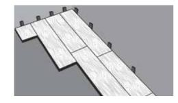
10. Measure the cut size for the final row and ensure you allow for the expansion gap. While fitting the final row, you may need the pull bar to ease the piece into place.
