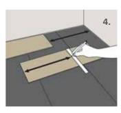
5. To cut the plank, use a simple utility knife and straight edge, and with the top side facing up, cut heavily and several times on the same axis. The knife will not go through the surface but make a deep cut. You can then lift one half of the plank using your other hand to hold down the second placing it very close to the cut. The plank will split naturally.
