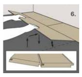
7. Click the long side of the plank into the previous row and place it tight to the short end of the previous plank with an angle of 30°. Drop the plank and gently press down the end with a rubber mallet so it firmly locks into the previous plank until both are at the same height. Make sure both planks are perfectly aligned.
