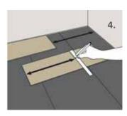
5. To cut the plank, use a simple utility knife and straight edge, and with the top side facing up, cut heavily and several times on the same axis. The knife will not go through the surface but make a deep cut. You can then lift one half of the plank using your other hand to hold down the second placing it very close to the cut. The plank will split naturally.
