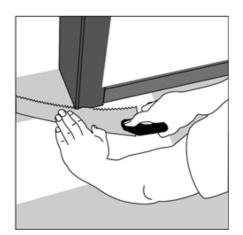
Helpful Hint: When installing each new row, take a full loose plank and use the long side to tap against the prior row to ensure no gapping.
